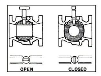
perpendicular to the ends of the valve, and flow is blocked.
