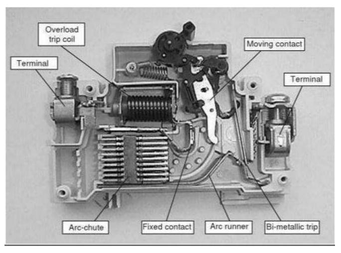
A circuit breaker contains an element that heats, bends and triggers a spring which shuts the circuit down. Once the element cools, and the problem is identified the breaker can be reset and the power restored.
