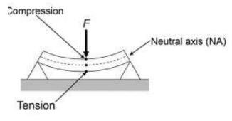
Simple supported beam bending
