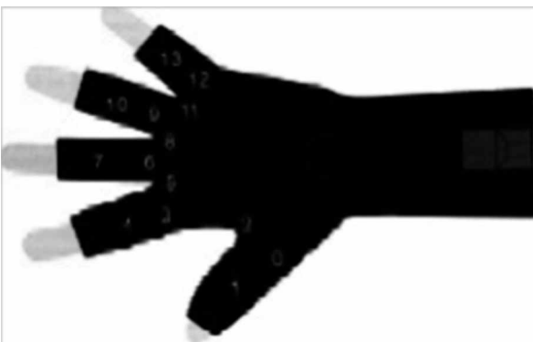
Figure 4. Sensor mappings for 5DT data glove 14 ultra
