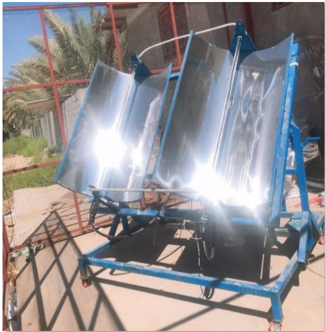
Solar collector This effort focused on the design and manufacture of an equivalent solar thermal collector. The aim of this work is to study the conversion of incoming solar energy into thermal energy to achieve some important applications in the use of solar thermal energy.
