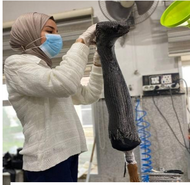
Manufacture of prosthetic legs from carbon fibre
