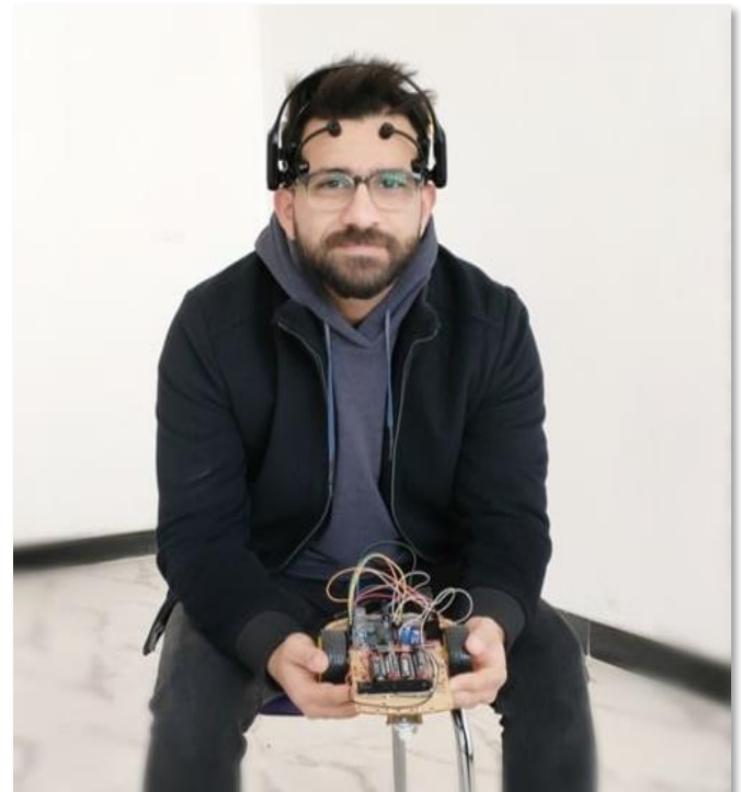
A wheelchair control system using a brain computer interface.
