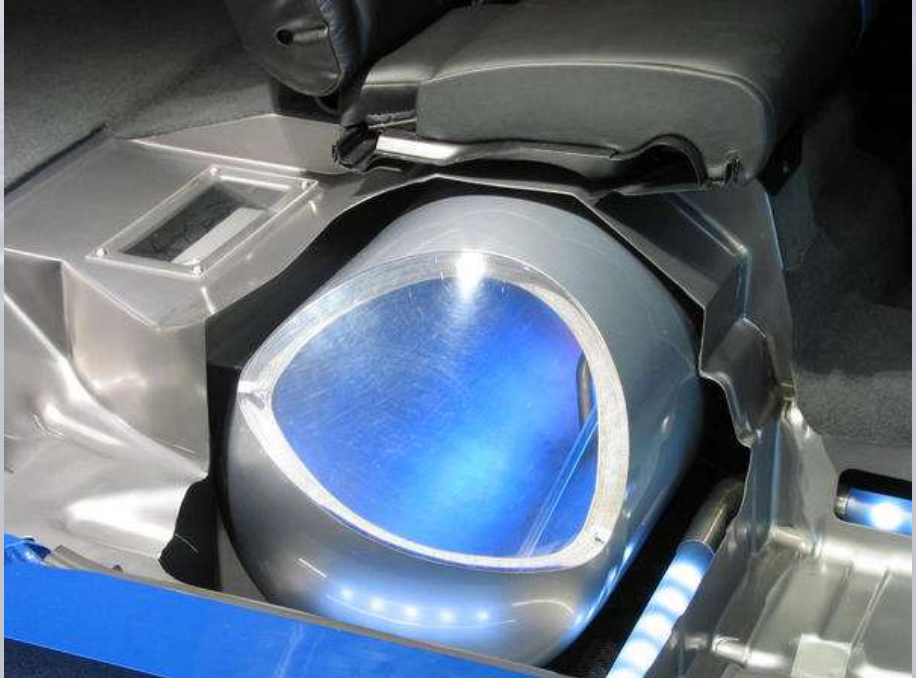
Fig. Liquid hydrogen tank for a hydrogen car
